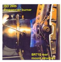
In the UK, the standard fire-test required by the Civil Aviation Authority (CAA) is performed under a procedure specified by the ISO report ISO2685 (1992). A propane-air burner is widely used in the UK to certify critical engine components exposed to the danger of fire in an aircraft engine. The alternative, Kerosene burner, which is frequently used in the US, is also specified in ISO2685 (1992) and in FAA report AC-20-135 (1990). An
